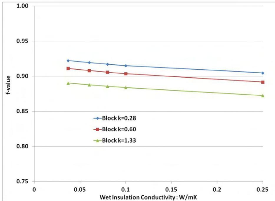
**Figure 16 – Calculated f-values for the solid floor**
