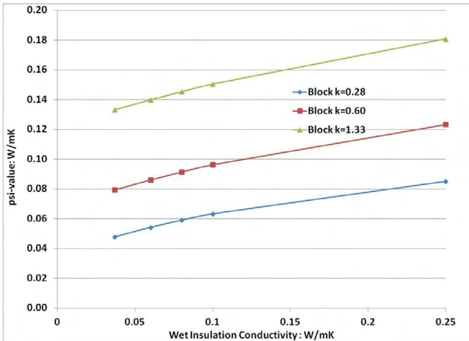
**Figure 15 – Calculated  $\psi$ -values for the solid floor**
