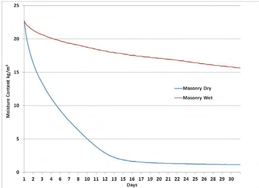
**Figure 22 – Mineral wool moisture content over 31 days after flooding, with the masonry initially dry or wet.**
