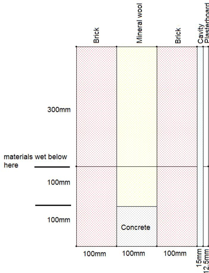
**Figure 17 – Materials and dimensions of WUFI model of cavity wall**
