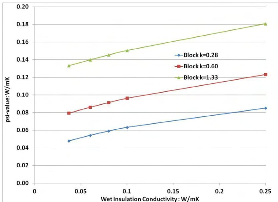
**Figure 13 – Calculated  $\psi$ -values for the suspended floor**
