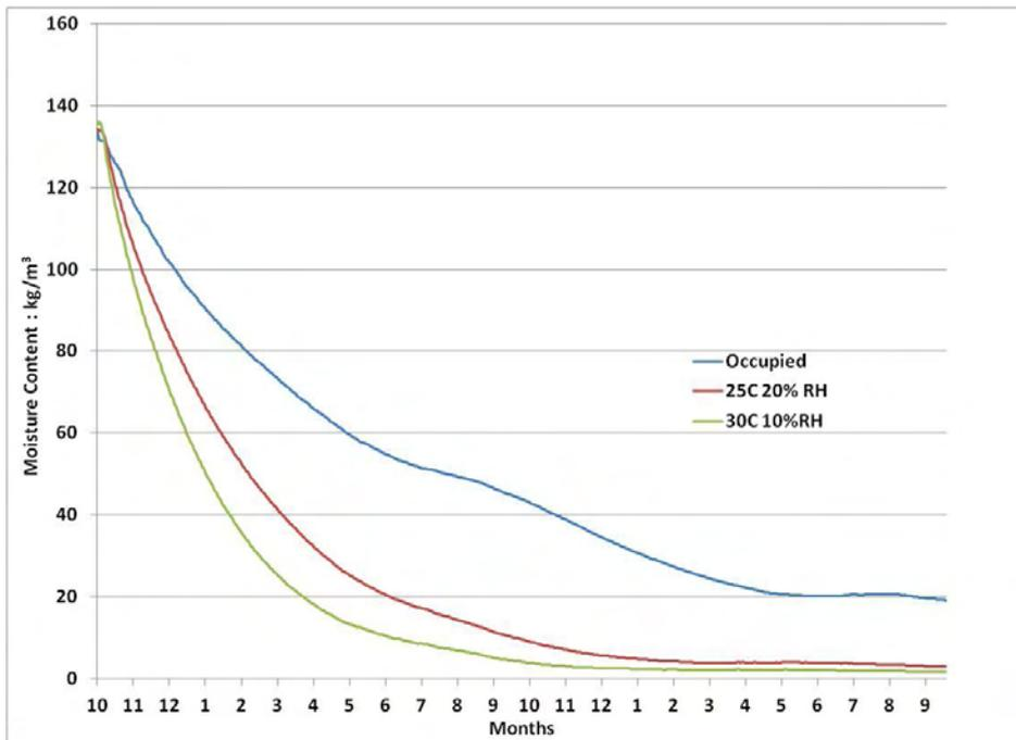
**Figure 24 – Inner leaf moisture content with house occupied and with two dehumidification regimes**
