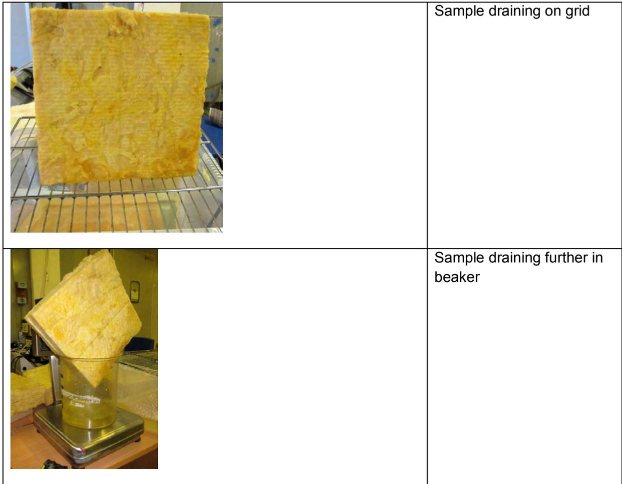
**Figure 9 – Sequence of images of small sample test**
