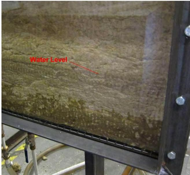
Figure 4 – Water level and wetted insulation as tank filling
