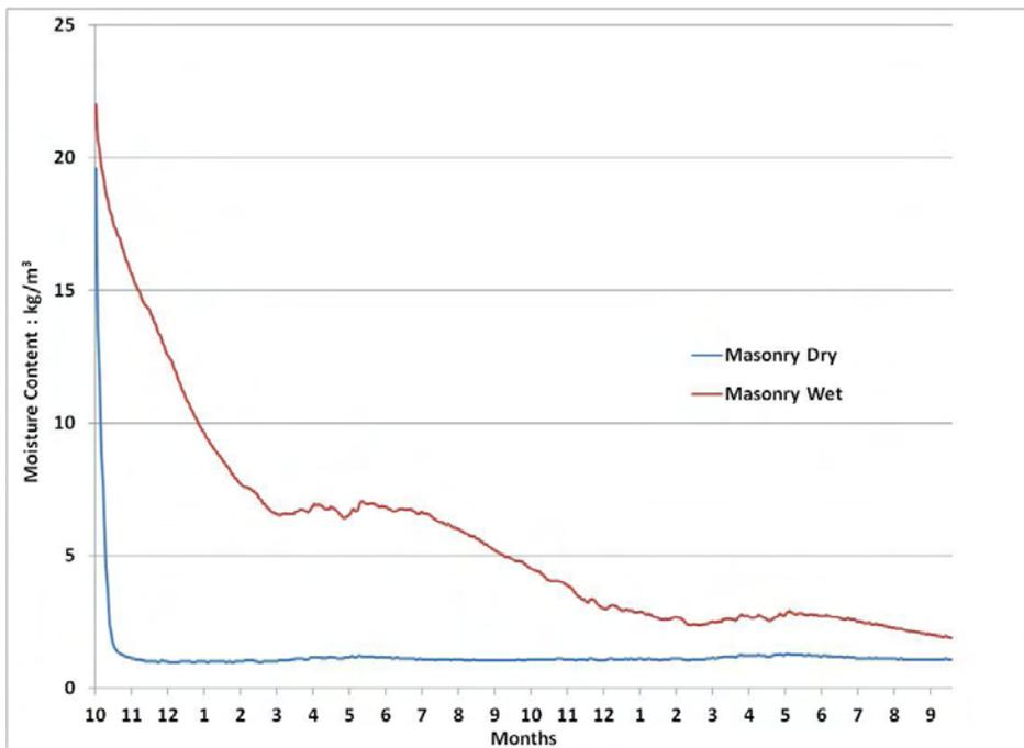
**Figure 23 - Mineral wool moisture content over 2 years after flooding, with the masonry initially dry or wet.**
