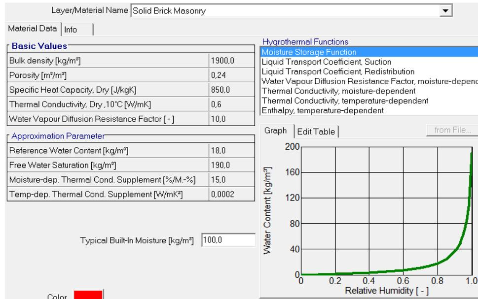
Figure 18 - Properties of brick from the WUFI database
