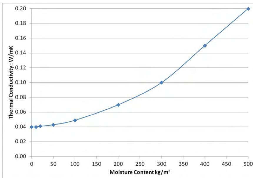
**Figure 11 – Thermal conductivity of mineral wool against moisture content (WUFI database).**
