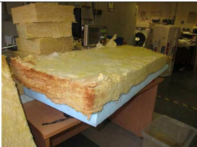
Bottom batt removed from the tank after being stood on end
