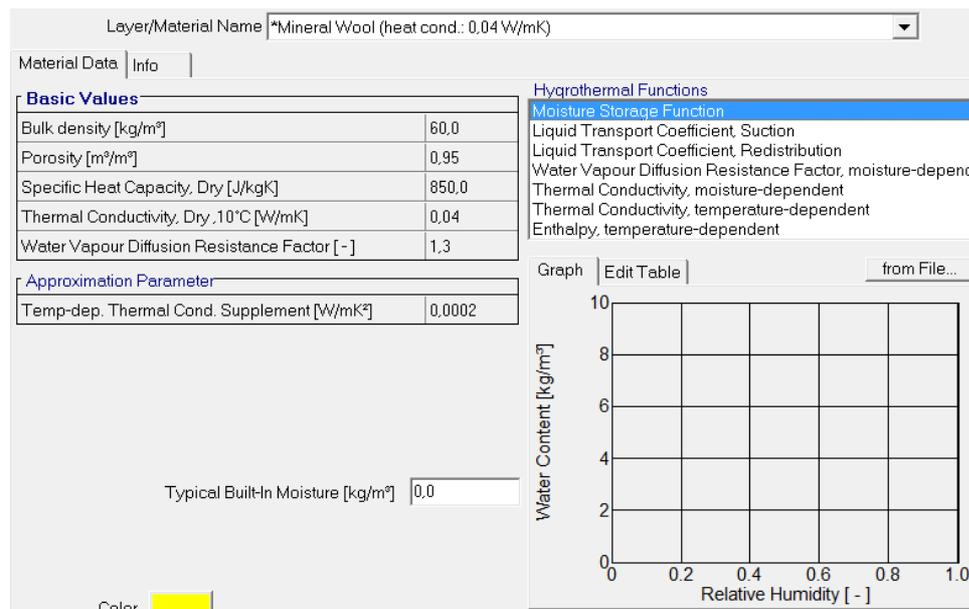
**Figure 19 – Properties of mineral wool from the WUFI database**
