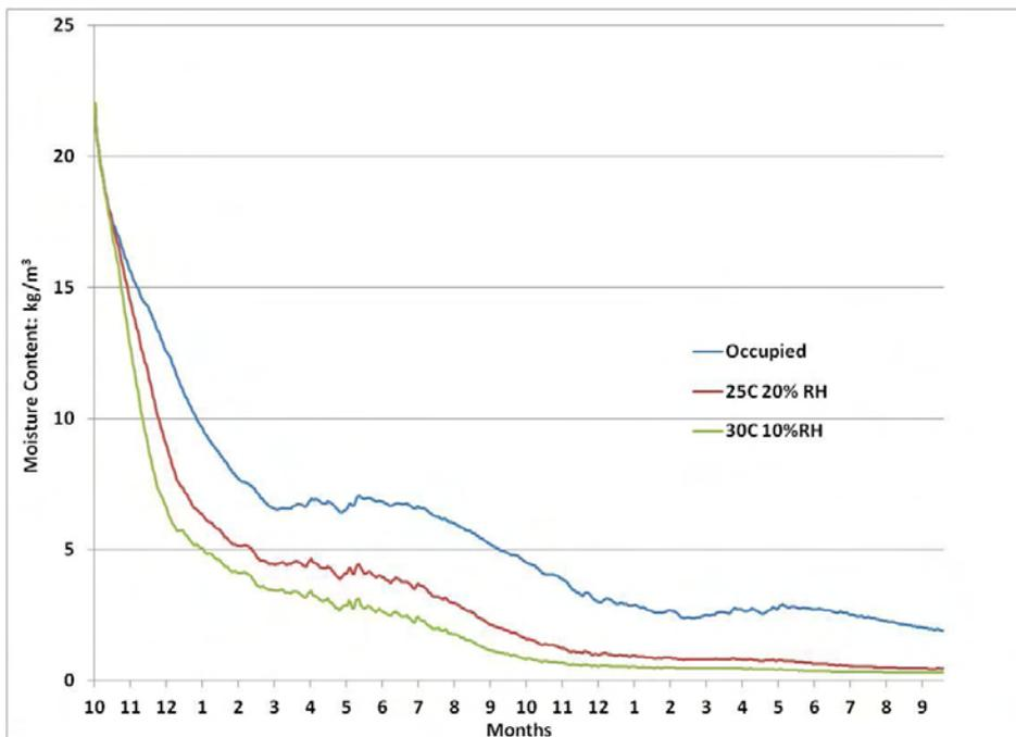
**Figure 25 – Insulation moisture content with house occupied and with two dehumidification regimes**
