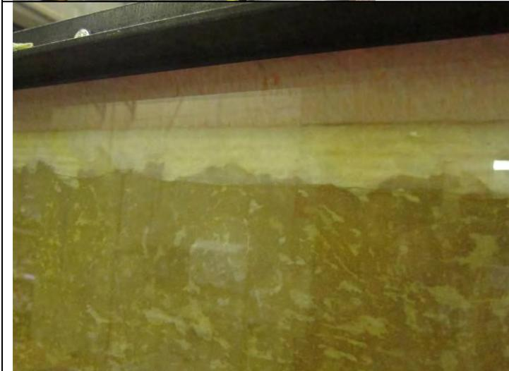
After 5 days of immersion, the water level has fallen slightly due to release of air
