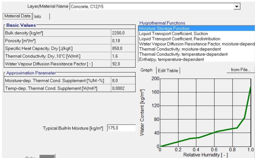
**Figure 20 – Properties of Concrete from the WUFI database.**
