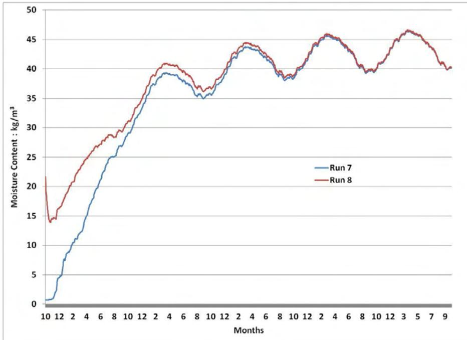
**Figure 21 – Base insulation moisture content, with rain turned on, for wall starting dry (Run 7) or starting wet (Run 8)**
